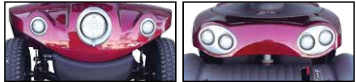
LED lighting system.
