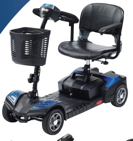
The Venom has many new features which are only normally found on larger scooters. It's the first Drive mini scooter to include Delta Bars as standard, it also features the next generation Drive splitting mechanism.
